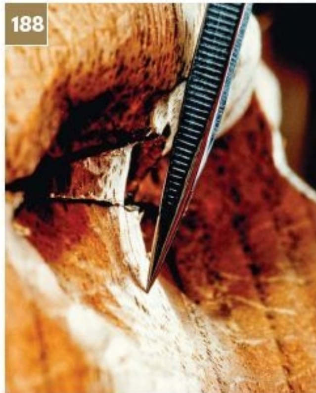
188 Sometimes this area can bulge out too far. If necessary, remove a little wood here.
