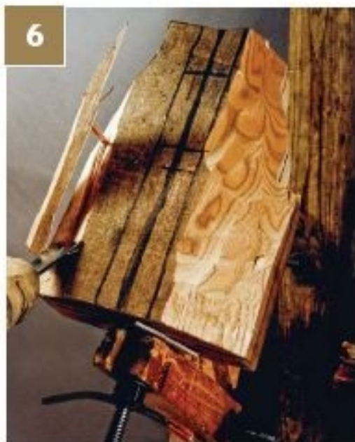
6 I work both sides of the block. The fishtail gouge quickly removes large pieces of wood.
