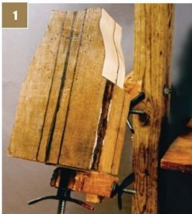
1 The first step is to cut out the front view using a band saw (pattern on page 32–33). Then I mark the centerline and lines 1" (25mm) away from the line on both sides.
