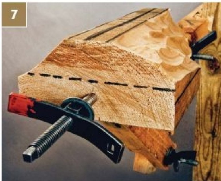
7 You can see the side of the blank has been wedged back and there is a flat spot down the center. Notice how the cuts relate to the guidelines I marked on the wood. These first cuts are beginning to give some shape to the piece.
