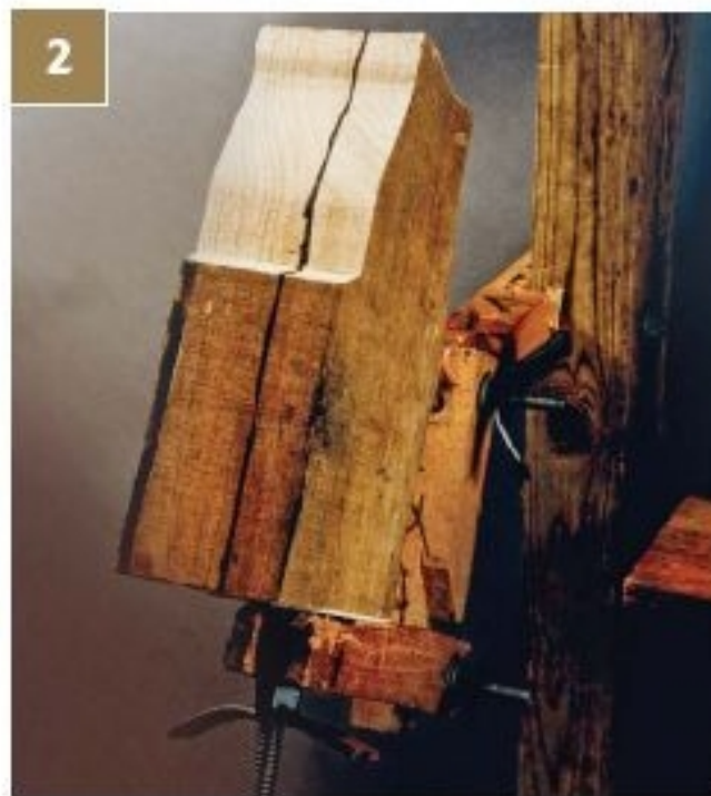
2 I turn the block to the side and mark a line 1" to 1½" (25mm to 13mm) in from the back of the block, running the length of the piece.
