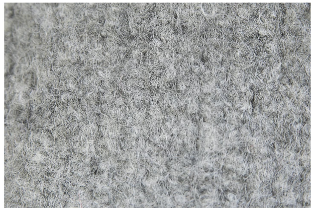
The same wool after felting. Most of the stitch definition is gone after just one felting cycle.
