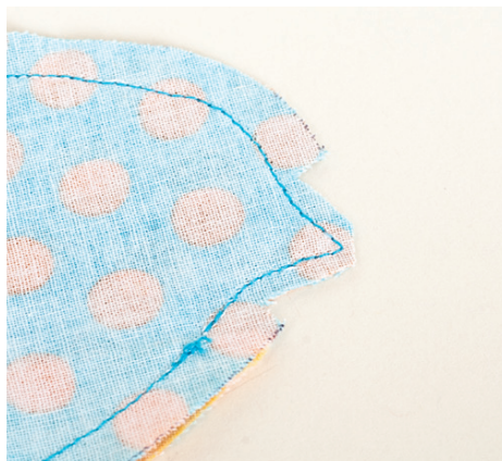
Clip inner points, trim seams to \frac{1}{8} ", and trim dog-ear at end of beak.
