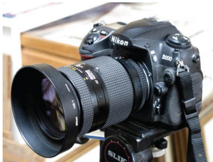
Fig. 10.4 A digital single lens reflex (SLR) camera. First choice for professional and keen amateur photographers, they can be very expensive, bulky and heavy. Advantages include an accurate through-the-lens viewfinder and interchangeable lenses making them still the best option for moving subjects and carefully composed and timed photographic shots. However, there are other options for photographing paintings.
