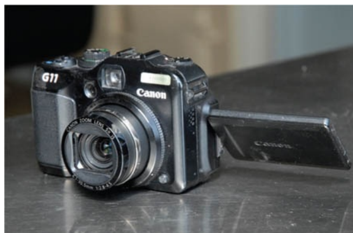
Fig. 10.5 Canon G11 compact digital camera. This compact is roughly a third of the size and weight of the Nikon SLR above. It has a viewfinder, which is of marginal use but it also has a swivelling screen, which is definitely helpful when photographing paintings. Image quality is excellent and as well as studio use, it's small enough to slip into a rucksack or pocket for general photographic work.
