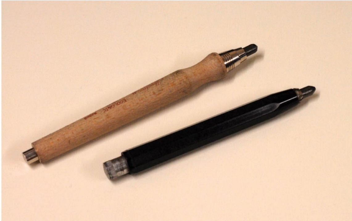
Fig. 3.6 Clutch pencils. A couple of examples of clutch pencils. The graphite lead is replaceable like a propelling pencil and is released or retracted by pressing the button on the end which protects it from breakage when clambering over fences and under barbed wire. They may appear clumsy at first but they're very versatile.
